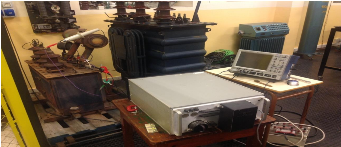
Figure.4-1 Experimental setup for transformer testing
