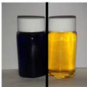
Figure 5.10. Photos of aliquots after complexation with CPC/CAS using DSh for the removal of external \text{LuCl}_3 after first washing (left) and 4 th final washing (right). The concentration of CPC/CAS is 0.2% w/v. The total volume of each fraction was 30 mL.
