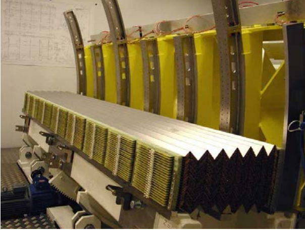
Figure 18: Photograph of a partly stacked barrel electromagnetic LAr module
