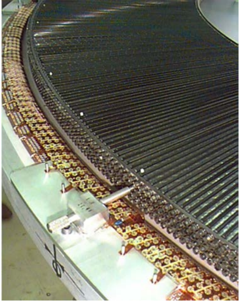
Figure 16: Photograph of four-plane TRT end-cap wheel during assembly. The inner and outer C-fibre rings can be seen, as well as the first layer of straws and the first stack of polypropylene radiator foils beneath it. Also visible are the plastic end-plugs which are used to position and fix the straws to the C-fibre outer ring. [22]
