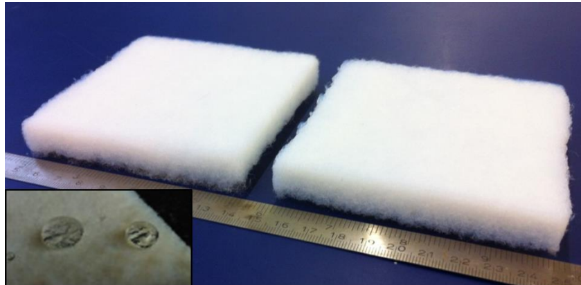
Figure 1: Digital photograph of the ambient dried PES-silica composite aerogels, inset shows the hydrophobicity of the composite
