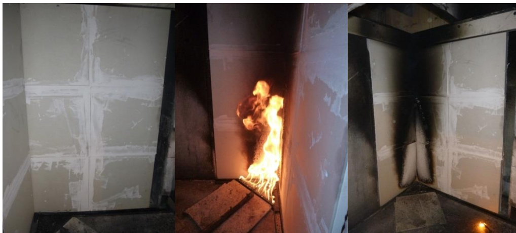
Figure 4: Images of the sample before (left), during (center) and after SBI test (right).
