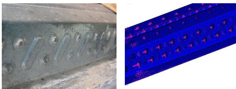
Figure 4.53 Traces of concrete and nodal forces
