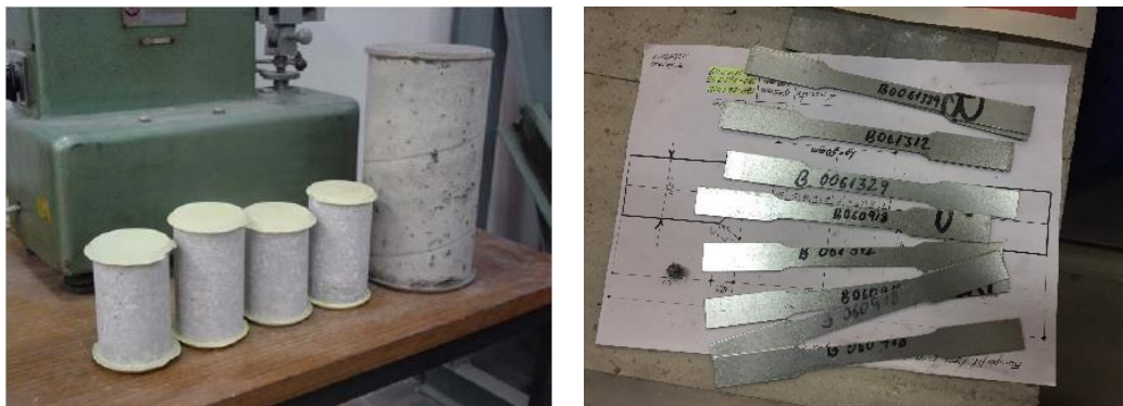
Figure 3.8 Concrete cylinders and steel coupons for material characterization
