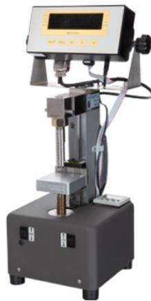
*Figura 17. Máquina Ultratester Bond Strength*
