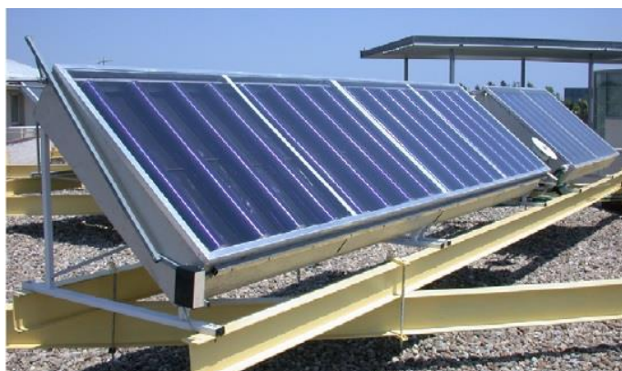
Figure 1.1. Prototype of a cascaded thermochemical process driven by solar thermal energy for deep-freezing [27].
