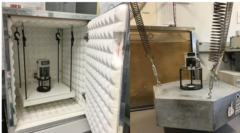
Figure 2.7. Two isolation systems are shown for the EC-STM. Both are based in the same concept of a platform (for the STM support) suspended from bungees (left image) or springs (right image).
