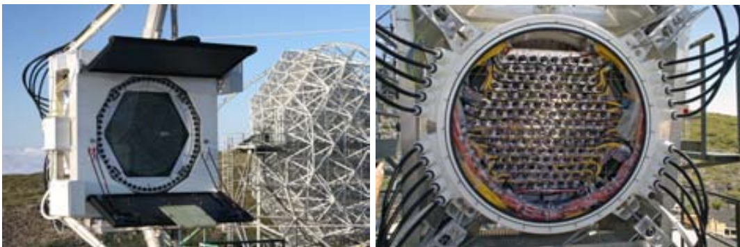
Figure 2.15: MAGIC II camera. On the left: photo of the camera from the front side. On the right: picture of the rear of the camera.
