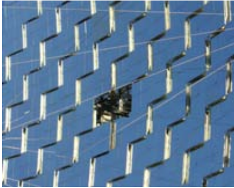
Figure 2.10: MAGIC I mirror staggering.
