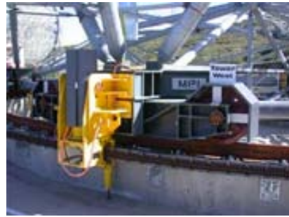
b) Azimuth motor sitting on a 2-wheel bogey
