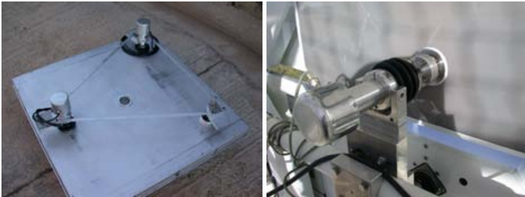
Figure 2.11: AMC motors. On the left: Picture of a mirror box from the back. The three mounting points, two of which with attenuators, are visible. On the right: Picture of an actuator fixed on the telescope frame.
