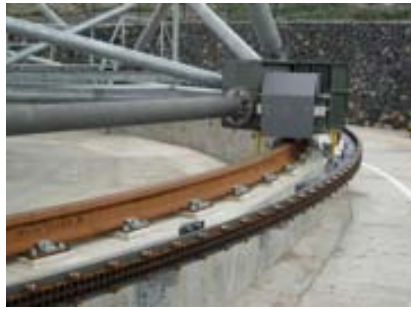
a) A detail of the azimuth drive chain and the azimuth rail
