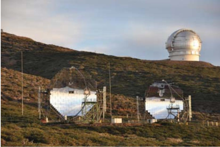
Figure 2.1: The MAGIC stereoscopic system of telescopes. On the left MAGIC I , operating since 2004. On the right, MAGIC II ended its commissioning phase in Autumn 2009. On the back ground , the Gran Telescopio Canarias, a 10.4 m \varnothing optical telescope also located the Roque de los Muchachos observatory.
