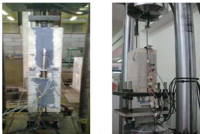
Figure 2.24: Test setups a) Double-shear b) Single-shear [91].
