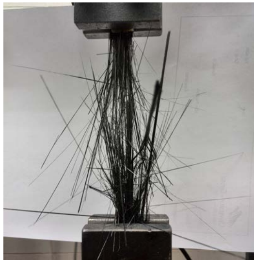
Figure 4.5: FRP rupture failure mode of CFRP laminates.
