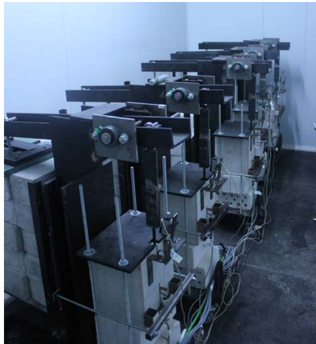
Figure 4.11: Long-term pull-out setup.
