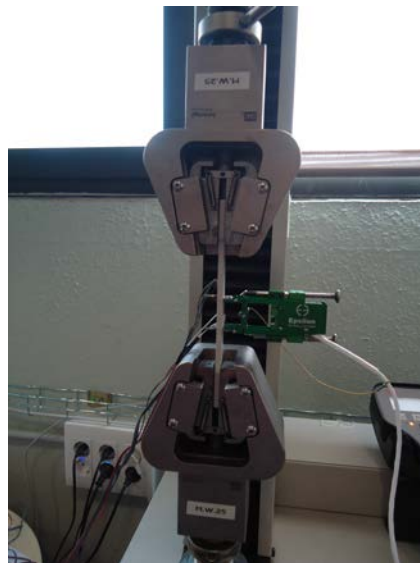
Figure 3.3: Tensile test setup and instrumentation.
