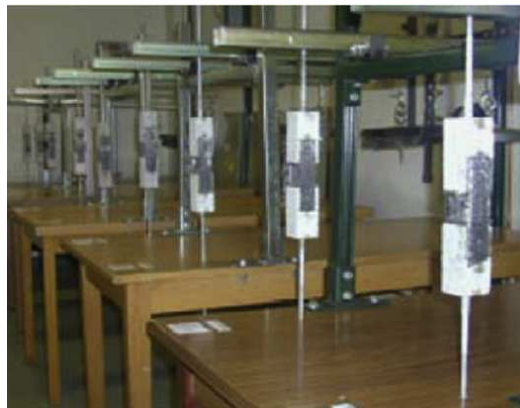
Figure 2.39: Double-shear test setup [130].
