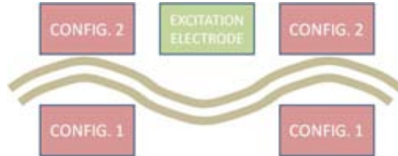
Figure 4.27: Schematic diagram of the bending profile and the location of output electrodes for the two configurations
