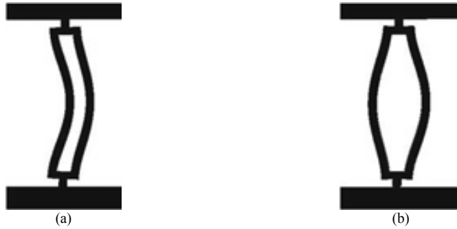
Figure A1.9: DETF lateral oscillation modes: (a) First lateral mode, unbalanced operation and (b) second lateral mode or balanced operation.
