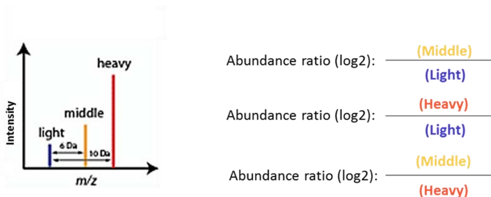
Figure 22: SILAC experiment with three cell populations labeled. Ratios between samples are calculated comparing the differences in the intensities of the peaks (adapted from (Geiger et al. 2011)).
