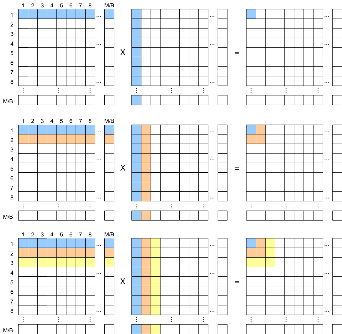
Figure 5-8: Schematic diagram of the grown in the granularity by the strategy of sending operands row/columns.
