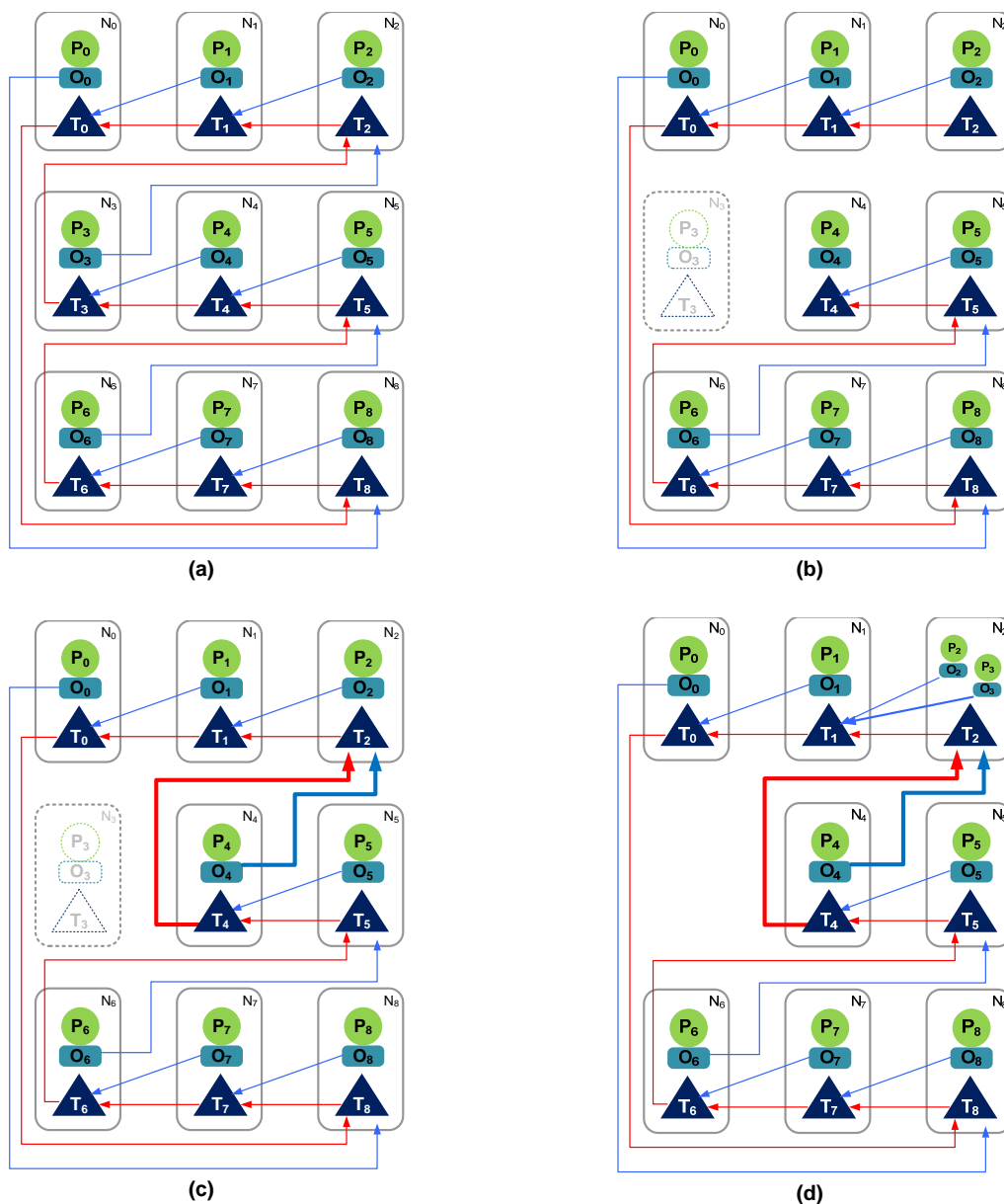
Figure 3-9: Recovering tasks in a cluster. (a) Failure free cluster. (b) Fault in node N 3 . (c) Protectors T 2 and T 4 detect the failure and reestablish the chain, O 4 connects to T 2 . (d) T 2 recovers P 3 /O 3 and O 3 connects to T 1 .
