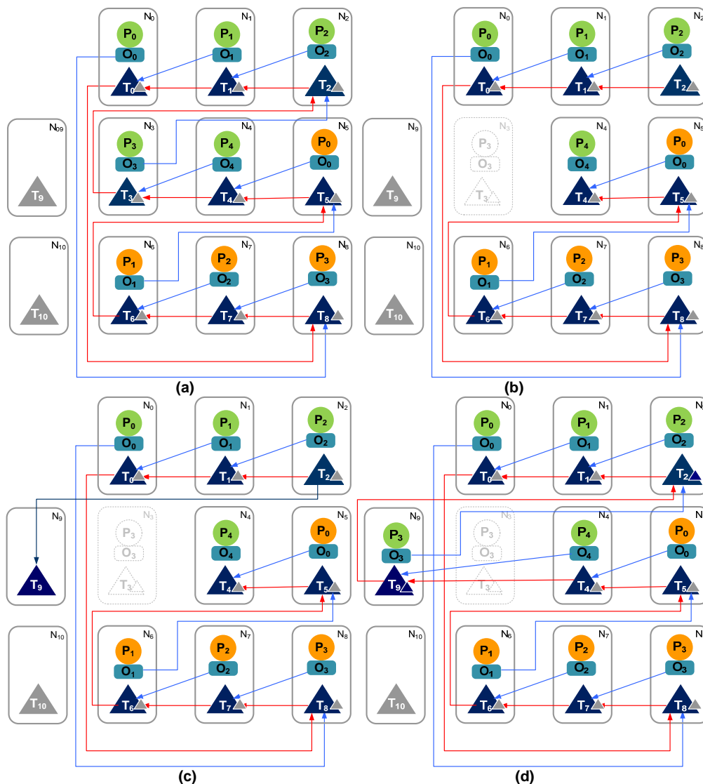
Figure 4-21: Recovering tasks in a cluster using spare nodes: a) before fault; b) N_3 fails; c) the spare is connected; d) P_3 recovers in the spare
