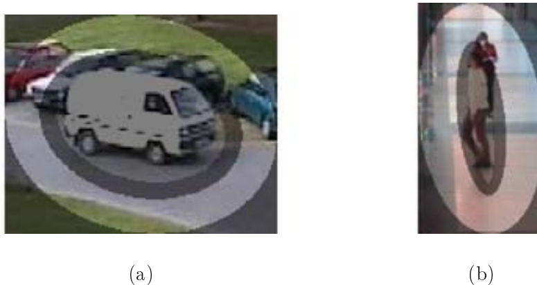
Figure 4.5: Examples of a centre-surround model with safety margin. (a) Tracked van from a traffic-monitoring sequence. (b) Tracked person from an indoor surveillance application in a shopping centre. Regions from centre to border: target estimation, safety margin, surrounding background, and non-local background.
