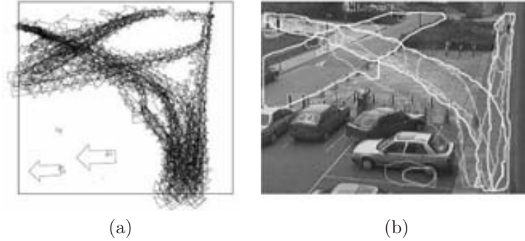
Figure 2.1: Early approaches on scene learning by trajectory analysis. (a) The neural network approach by Johnson and Hogg [58] (b) Semantic regions obtained by Fernyhough et al. [39].
