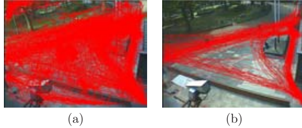
Figure 3.1: (a) Original trajectory dataset (4250 trajectories). (b) Trajectory dataset after removing tracking failure noise and semistationary motion noise [67].
