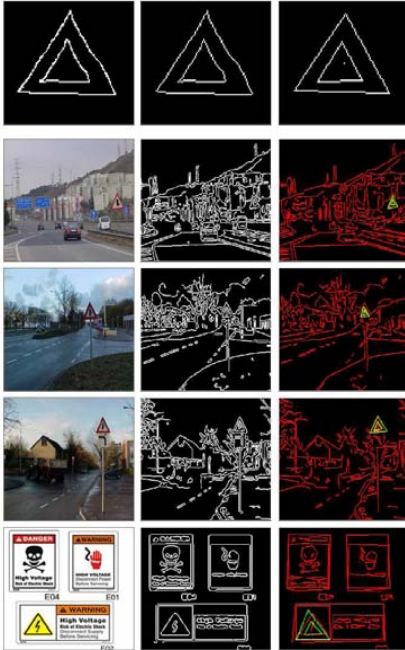
Figure 5.18: Example of sketch detection: alert sign. From top to down, the T values of the matching are: 0.69, 0.70, 0.76, 0.72
