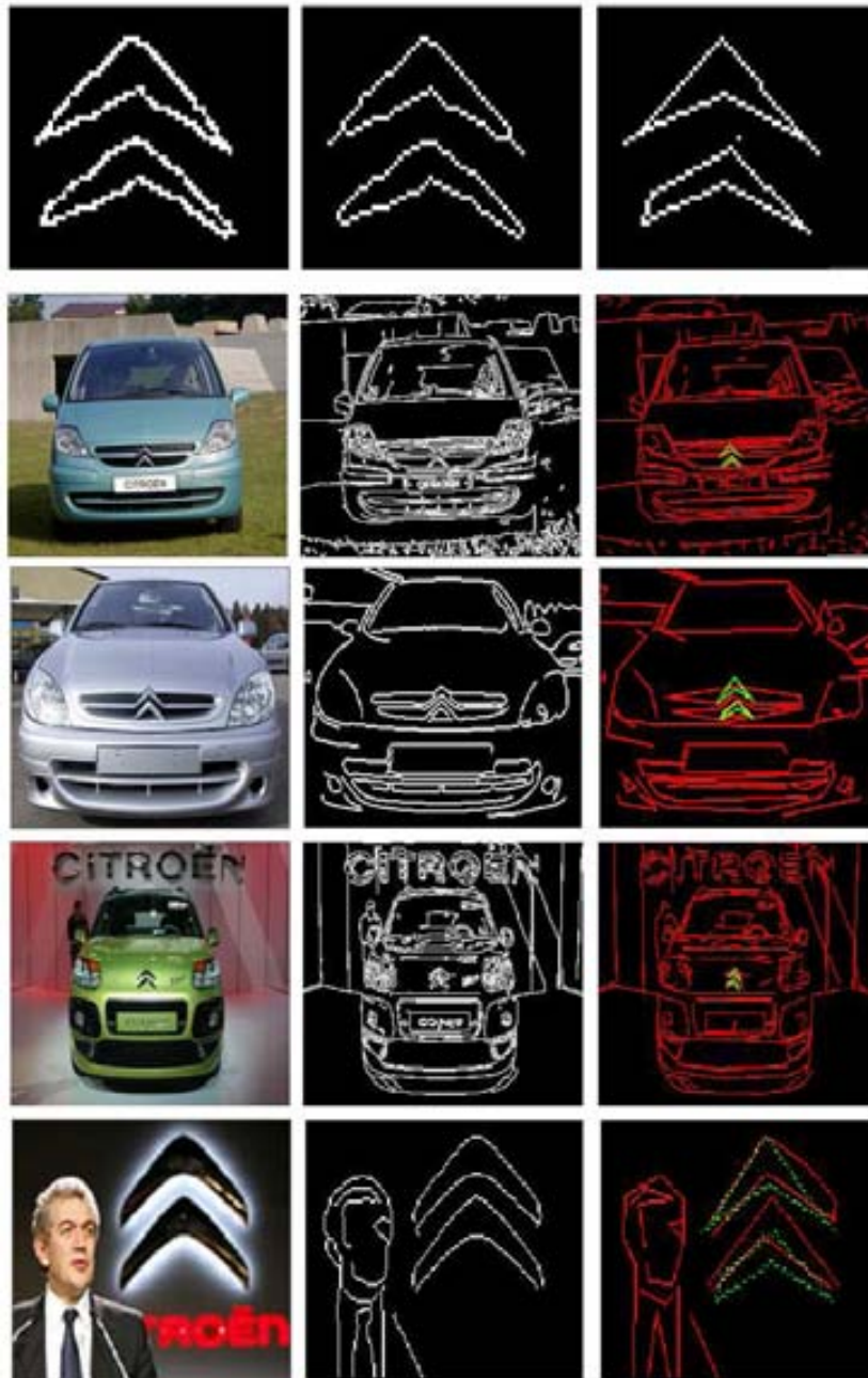
Figure 5.17: Example of sketch detection: car logo. From top to down, the T values of the matching are: 0.77, 0.75, 0.75, 0.68.
