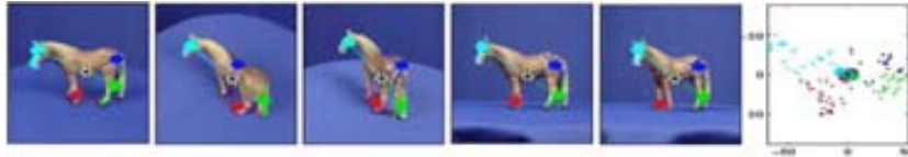
Figure 2.36: The image of a horse is modelled by the average position of the subparts according to different points of view. A generalized Hough voting strategy accumulates the evidence of the object detection in a hierarchical structure of three levels (reprinted from [BT05]).
