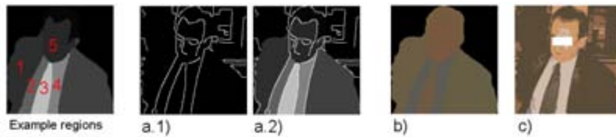
Figure 4.7: Example regions n_1, n_2, n_3, n_4, n_5 . a) Boundary Distance: BD(n_2, n_2)=1 , BD(n_4, n_5)=0.9 , BD(n_2, n_5)=0 . b) Average Color Distance: ACD(n_2, n_4)=0.2 , ACD(n_1, n_2)=0.68 . c) Color Histogram Distance: CHD(n_2, n_4)=0.12 , CHD(n_1, n_2)=1 .
