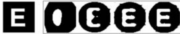
Figure 2.21: Example of the reconstruction of the left image with the Zernike moments of order 5, 10, 15 and 20.
