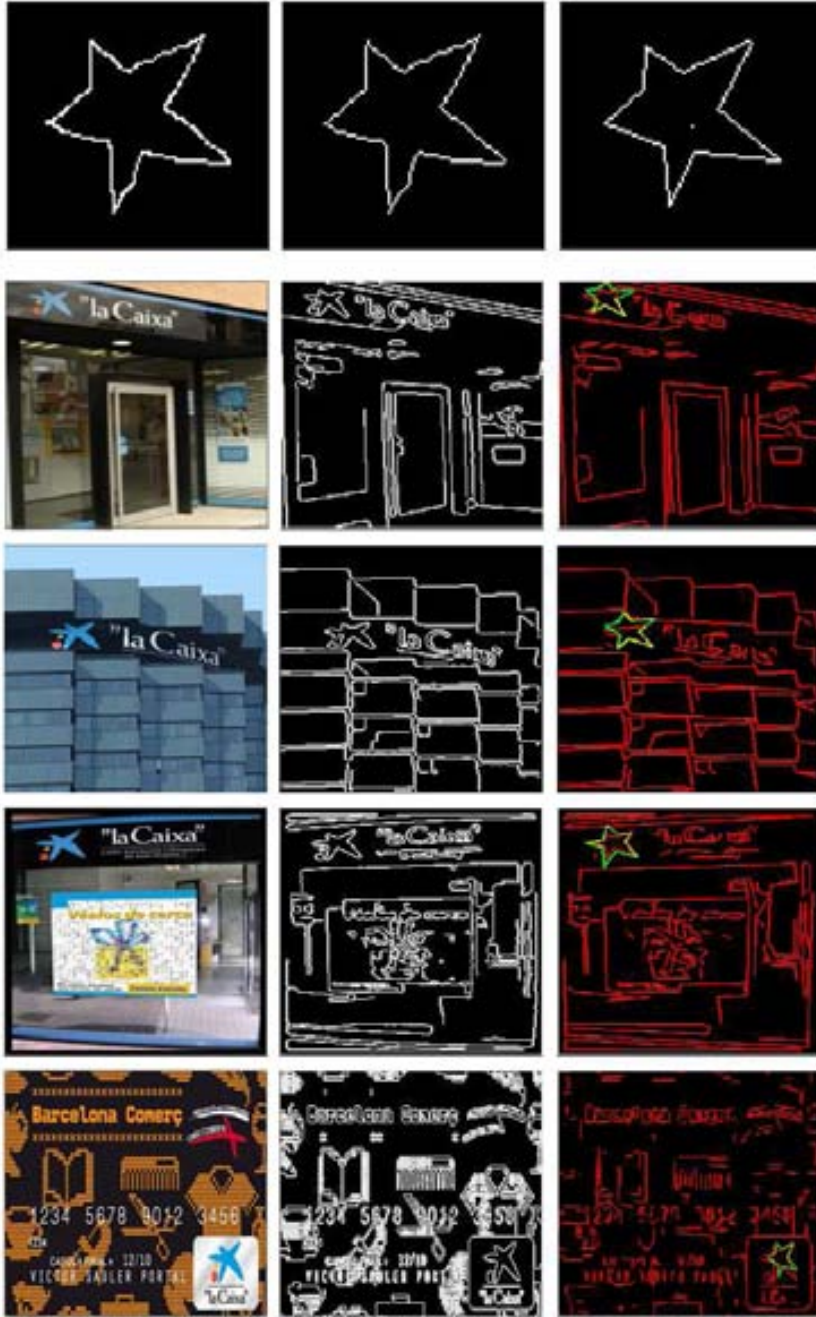
Figure 5.16: Example of sketch detection: star. From top to down, the T values of the matching are: 0.63, 0.70, 0.64, 0.69
