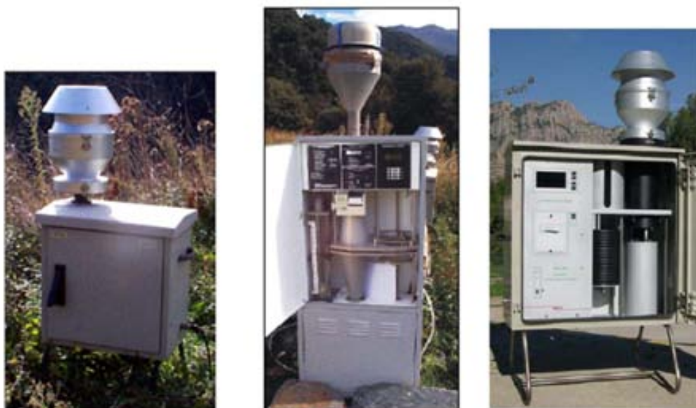
Figure 3.10. MCV-CAV high volume sampler (left), DIGITEL DH-80 sequential high volume sampler (center) and MCV CAV-A/M-S sequential high volume sampler (right).
