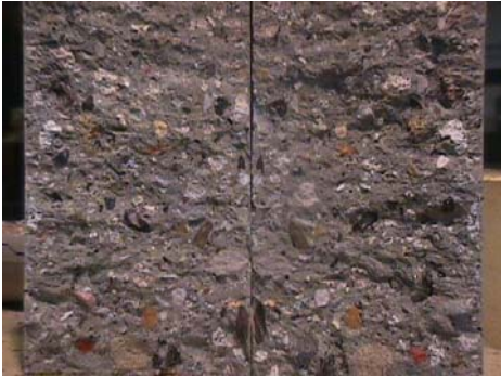
Fig. 3.10: Recycled aggregates concrete failure way by tensile
