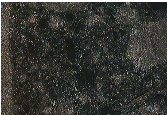
Fig. 4.21: Portlandite distribution in HC. White shining points are portlandite crystals. Width of field 0,5 mm
