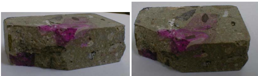
Fig.4.5: Recycled aggregates are not carbonated. The rose colour shows that the alkalinity of the aggregates.
