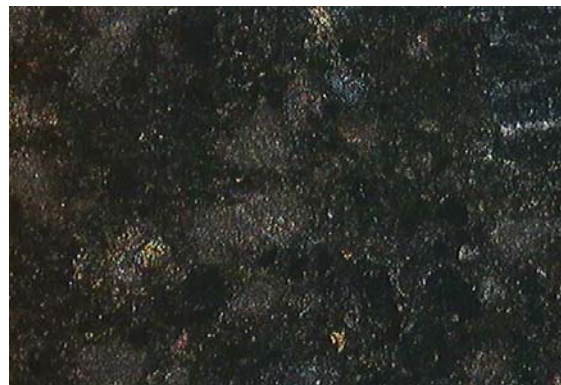
Fig. 4.22: Portlandite distribution in HR100. Width of field 0,5 mm
