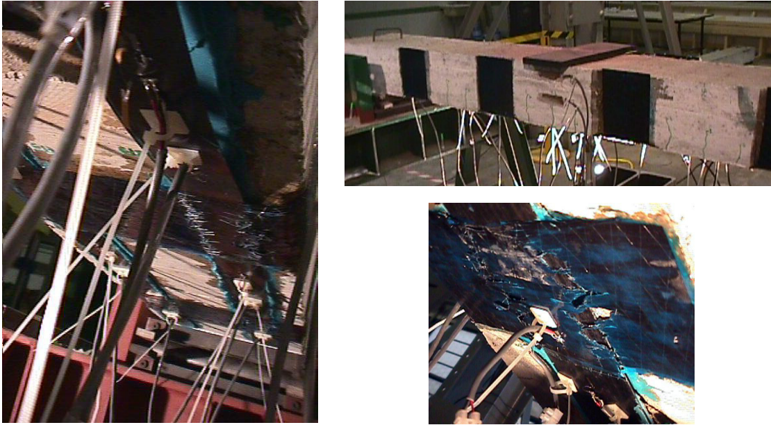
Figure 2.5. Test set-up for Beam 2/B with full-height plies of carbon sheet as external anchorage. Sheet rupture after laminate peeling in Beam 2/A (right side) and 2/B (left side).
