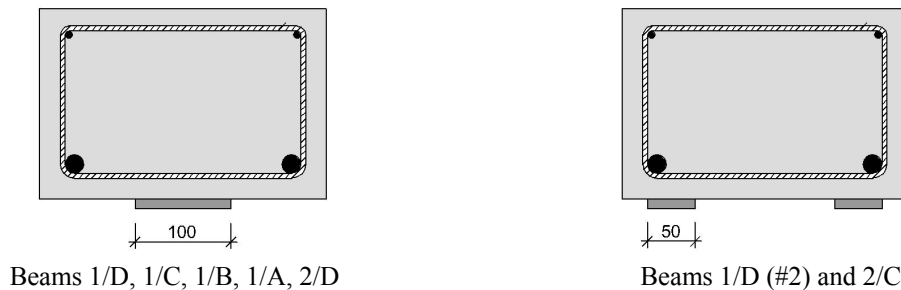
Figure 2.4. Beams 1/D, 1/C, 1/B, 1/A and 2/D sections vs. 1/D (#2) and 2/C. (Dimensions in mm)
