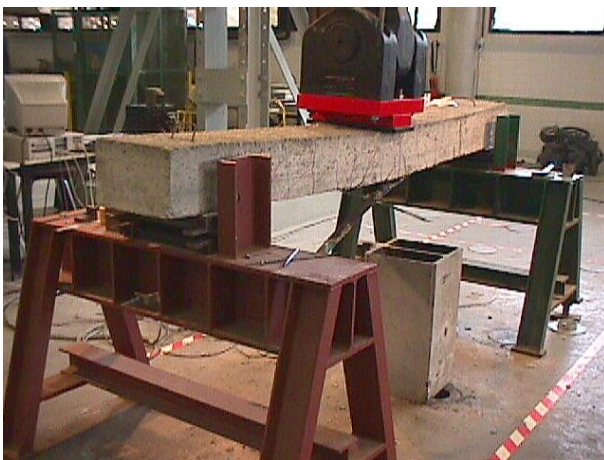
Figure 2.2. Test set-up for Beams 1 and 2.
