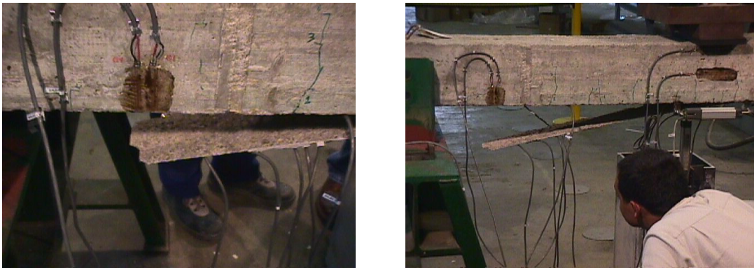
Figure C.12. Peeling failure in Beam 1/D due to a lack of anchorage.
