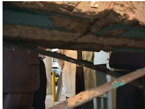
Figure C.67. Debonding of both laminates at the end of the test. Peeling may have initiated due to an intermediate existing crack that appeared during the first failure test of Beam 1/D.
