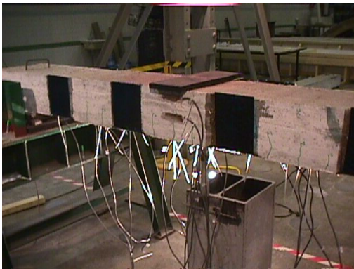
Figure C.53. Crack pattern at service and at failure load, and instrumentation affixed to Beam 2/B.
