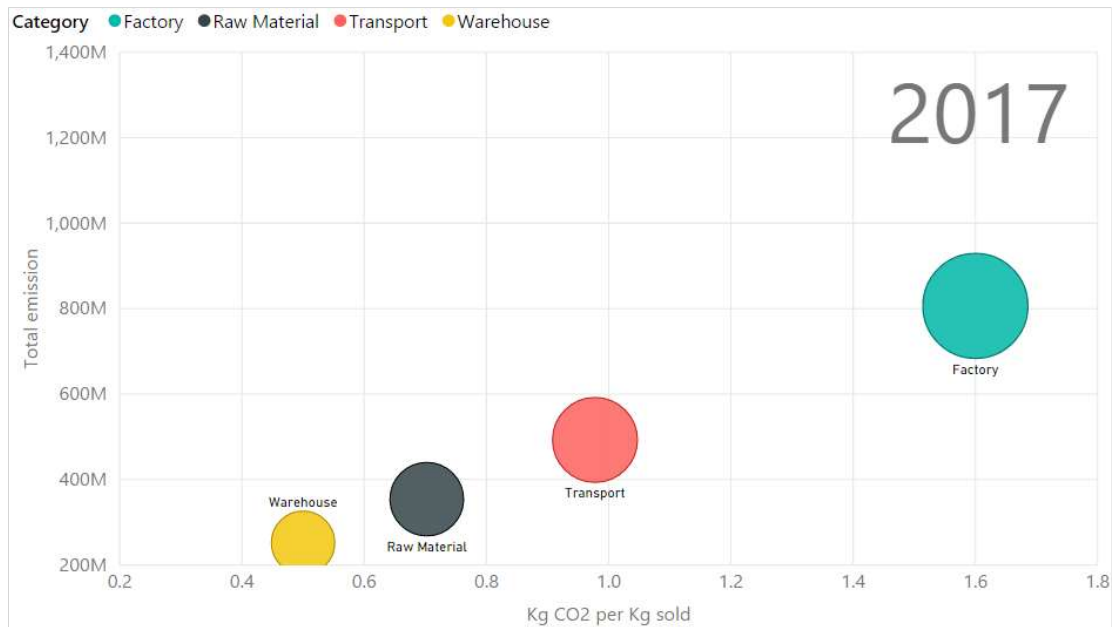
Figure 7-16 Initial situation of the Kg CO 2 e per Kg sold rate. Source: Own preparation
