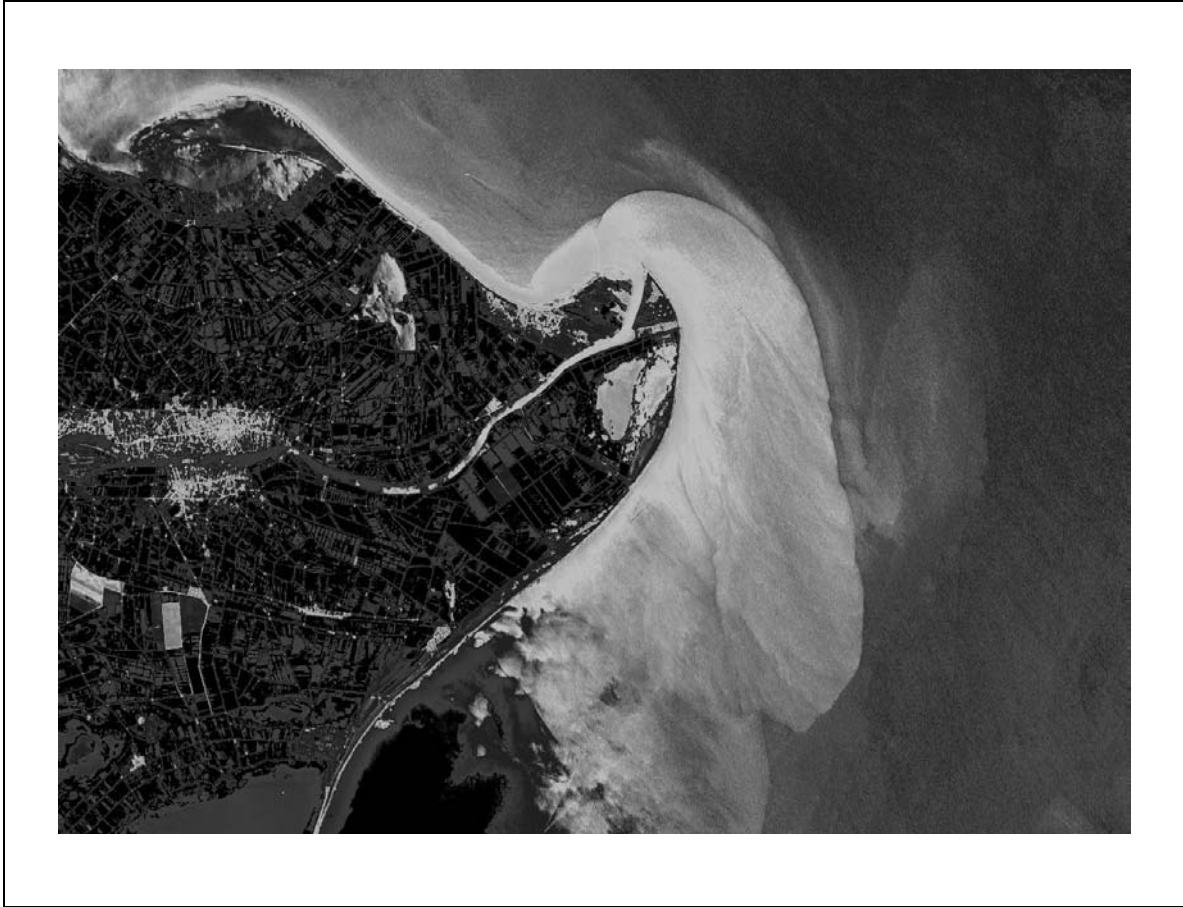
Figure 6.40: Satellite image of the river Ebre's freshwater plume, on July 6th, 1997, at 11:03 UTM. The colour scale refers to extra-atmospheric radiances measured by SPOT, HRV sensor, XS2 channel ((c) CNES).
