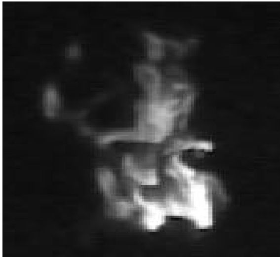
Figure 4-45.- Example of a dye introduced into a grid stirred turbulent flow. If the structure of the dye is to be analysed and compared with the structure of the turbulent flow, two methods will be needed.
