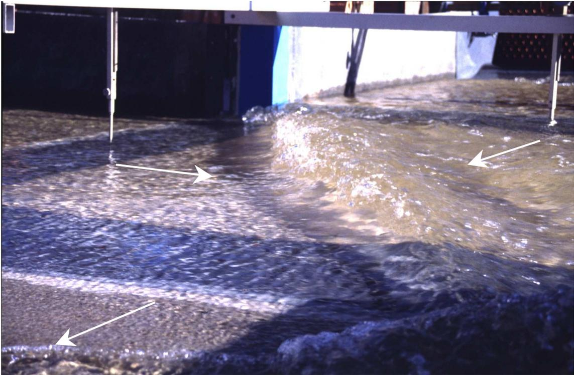
Figura 6-6: Resalto débil.  $Q_{ex} = 99,7$  l/s;  $Q_{ey} = 25,0$  l/s;  $Q_{sx} = 97,3$  l/s;  $Q_{sy} = 27,4$  l/s;
