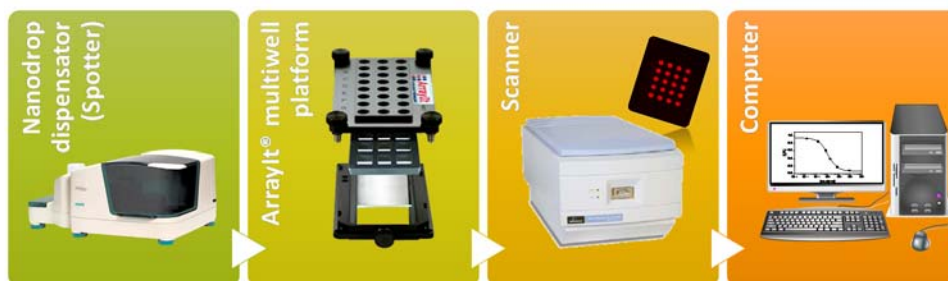
Figure 5.5. All material needed for the different steps involved in fluorescent microarray development: print, assemble, measure, analyze and data treatment.
