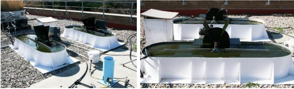
Figure 3-7. Experimental high rate algal pond (laboratory of the GEMMA research group, Barcelona)
