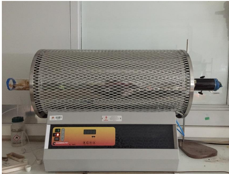
Figure 2.9 Tubular furnace used for heat treatment processes
