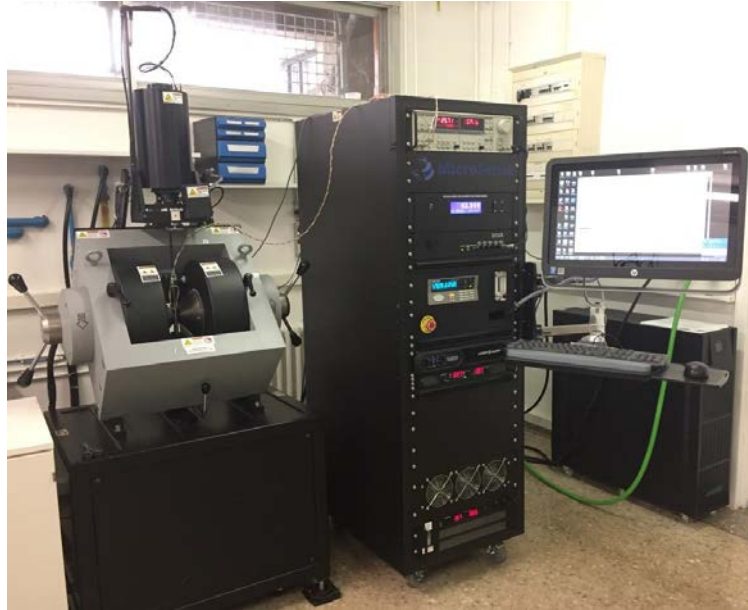
Figure 2.17 The VSM equipment used
