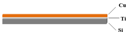
Figure 2.4 Scheme of Si/Ti/Cu substrate used for bismuth ferrite electrodeposition
