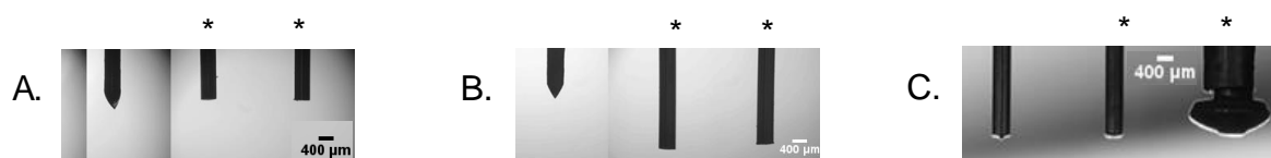
Figure 3.7. Configurations of array-end electrodes used in this study. Such electrodes are marked with a *, while the spraying needles show Taylor cones. The end electrode configuration is symmetric for both ends of the LEsS (right side shown). Emitter diameter (D) is 400 μm.
