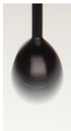
Figure 3.3: Time evolution sample stack of pictures of the pendent drop (10 sec intervals), that was used to estimate the volume and subsequently the volumetric flow rate using ImageJ software.
