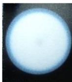
Figure 3.5: A single needle deposition spot top-view, when no other emitters are operated at close proximity. Q=2\mu\text{l}/\text{min} , RH=40.1 percent, T=20.4 C, H=22 mm, solution BREC. Single emitter setup, applied voltage= 6.1 kV.
