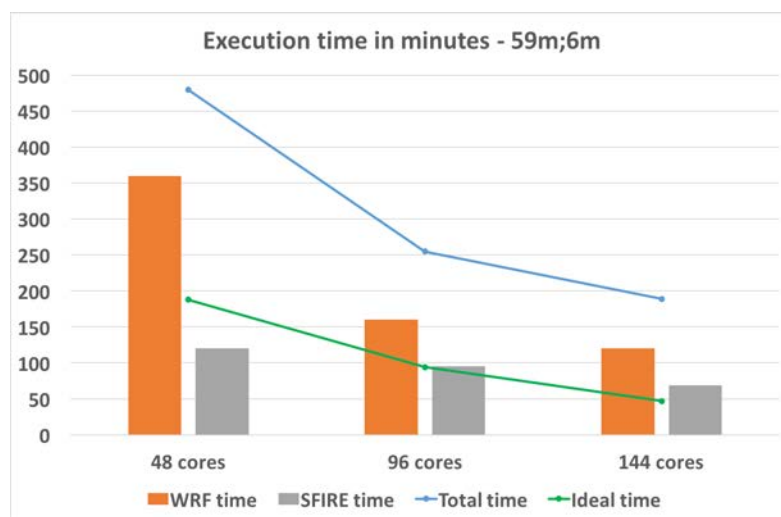
Figure 3.9: Ideal, WRF, SFIRE and total execution time in minutes simulating the Cardona fire using WRF-SFIRE with an atmospheric grid resolution of 59 meters and MPI parallelization with 48, 96 and 144 cores.
