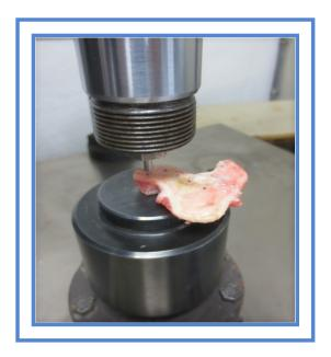
Figure 28. Bionix 358 servo-hydraulic mechanical test machine (MTS, USA)
