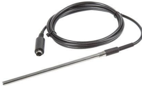
Figura 3.4 Sensor de temperatura RTD Desin, model PT100.
