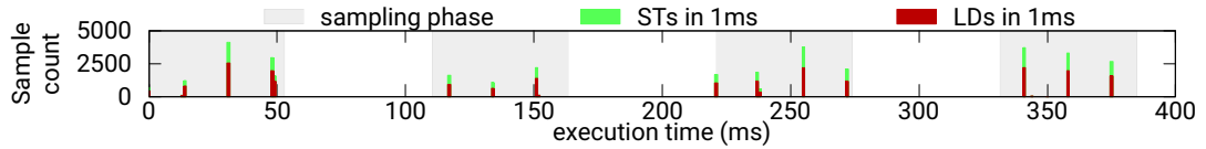
Figure 6.8: Number of recorded samples per millisecond over time, summed over all threads, running using 8 threads
