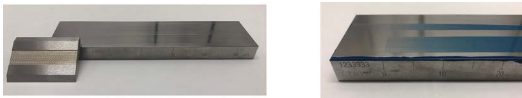
Figure 5.3: Grind gauge used for the estimation of particles size in a screen-printing paste. The appearance of grooves in the pass indicates the size of the particles mixed in the paste.
