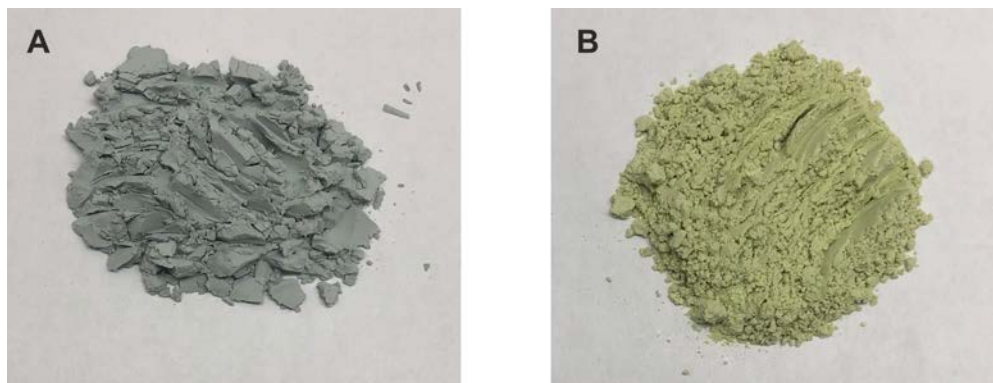
Figure 5.2: Image with the powders of the two tin oxide-based particles used for the modification with Prussian Blue. (A) SiO 2 -ATO, (B) ITO.
