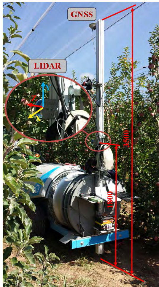
Fig. 1. View of the MTLs equipment showing the GNSS antenna placement and the mounting orientation of the LiDAR sensor. Distance data are in mm.
