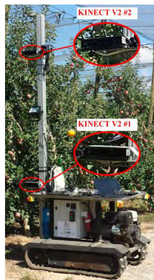
Figure 1. View of the acquisition equipment showing the Kinect v2 sensors mounted on the mobile platform.
