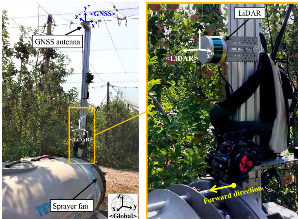
Figure 2. Global scheme of the experimental setup used for data acquisition. The orientation of \langle LiDAR \rangle , \langle GNSS \rangle , and \langle Global \rangle coordinate systems used for point cloud generation are represented.
