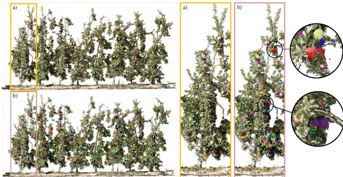
Figure 9. Illustration of 3D fruit detection and location results from the test dataset: a) 3D visualisation of the scanned scene. b) Test scene with coloured fruit detections. A zoom view is shown to assist the visualization of the detections in the first tree of the dataset. Black circles show two examples where two apples were unified in a single detection. The reader is referred to the following link for an interactive 3D visualization of test fruit detection results: http://www.grap.udl.cat/documents/photogrammetry_fruit_detection.html
