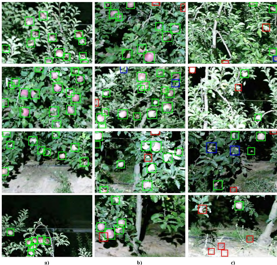
Figure 8. Fruit detection results on RGB_{nr}+S+D test set using anchor scales of 4, 8 and 16. True positive detections are shown in green squares, false positives in red and false negatives in blue. Images are ordered according to their F1-score. Column (a) contains examples of the best detection results, F1-score = 1. Column (b) contains the four intermediate scored images of the test set, corresponding to an F1-score = 0.91. Column (c) shows the worst detections, ordered from bottom to top with an F1-score = [0.23, 0.67, 0.67, 0.67].
