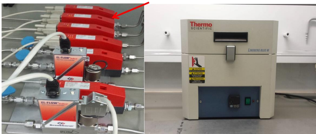
Figure 2.1. Growth system: The flow meters (right panel) and the growth furnace (left panel).
