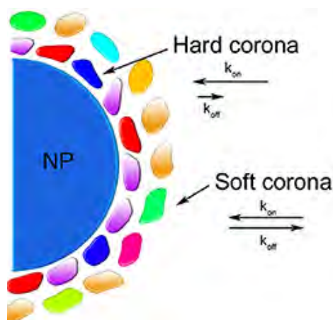
Figure 1. Formation of the NP-biomolecule corona 22 . Upon exposure to physiological fluids, NPs become coated with a variety of proteins and other biomolecules. The hard corona is comprised of lower abundance, high affinity biomolecules with almost negligible exchange rates. The soft corona is comprised of more abundant, lesser affinity biomolecules with faster exchange rates.
