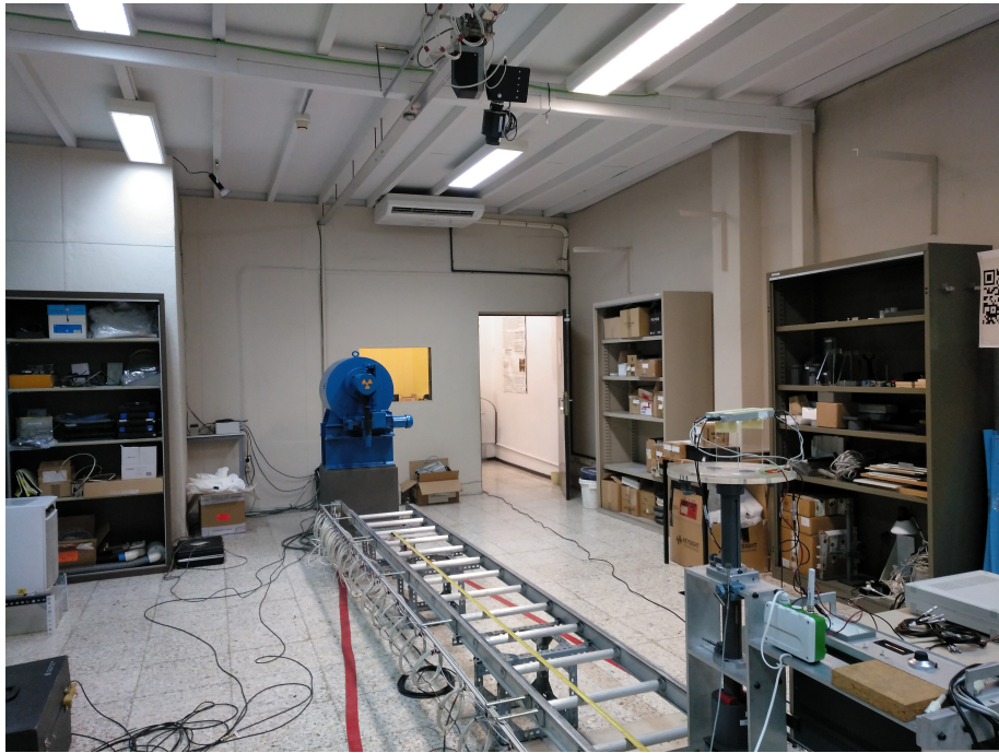
Figure 2.6: Photo of the experimental configuration at LCD. Detectors are placed on top of a rotary plate, which is 5 m away from the source.
