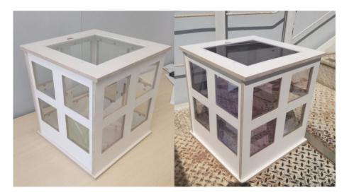
Figure 5-6: photograph of the photochromic glass-containing building model.
