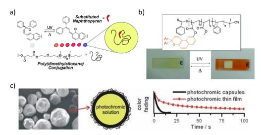
Figure 1-6: strategies that minimize the matrix effect: molecular functionalization with flexible polymeric tails (a),<sup>[63]</sup> embedment of the dye in low  $T_g$  polymeric matrices (b)<sup>[66]</sup> and encapsulation of the dye into liquid-core microcapsules(c).<sup>[82]</sup>
