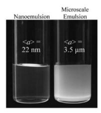
Figure 1-9: transparent nanoemulsion (radius = 22 nm) and opaque microscale emulsion (radius 3.5  $\mu$ m), at the same oil concentration in the water phase. [98]
