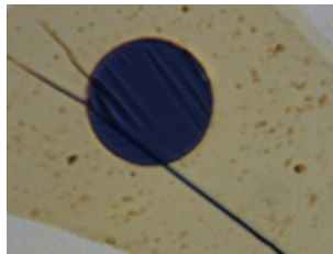
FIGURE 3.9: SAMPLE B - Optical microscope picture of suspended 7-layer MoS 2
