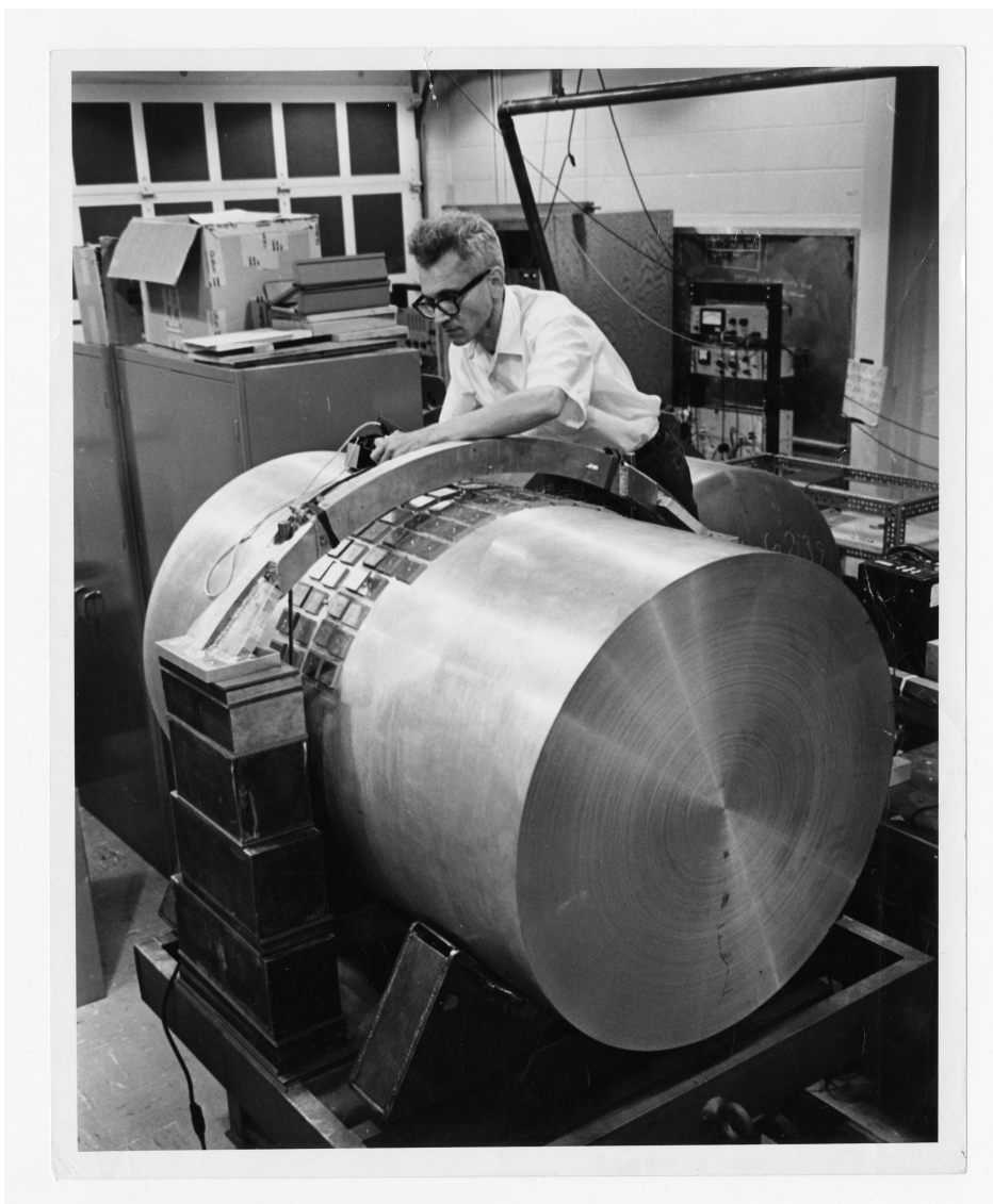
Figure 5: Professor Joseph Weber with a \text{GW} detector (Credits: Special Collections and University Archives, University of Maryland Libraries www.umdrightnow.umd.edu ).
