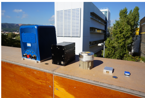
Figure 5.2: Image of a set of inertial systems: from navigation-grade to MEMS.
