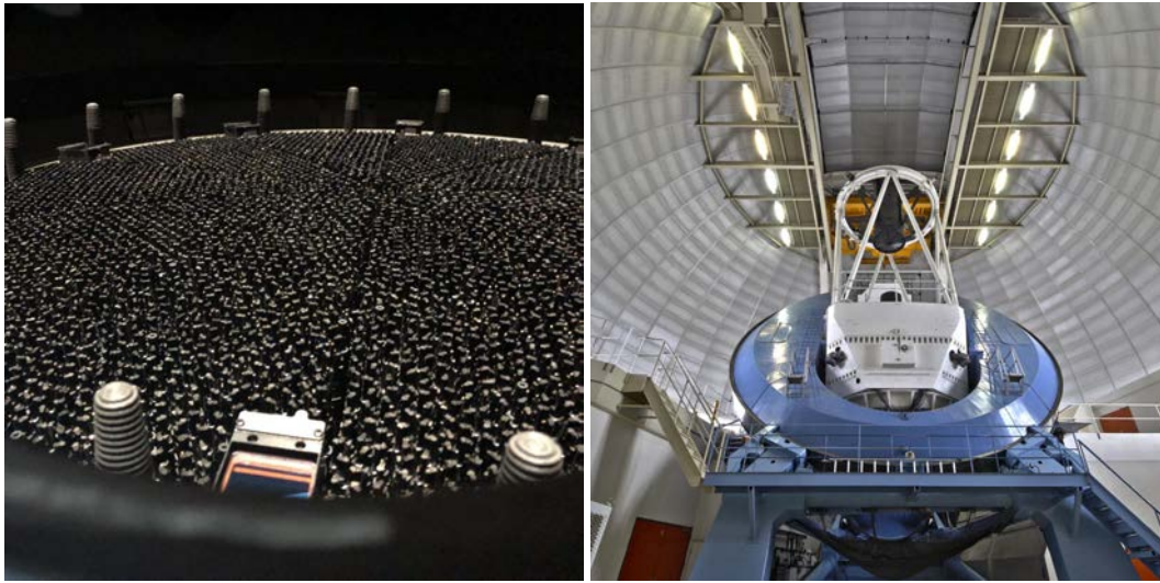
FIGURE 3.6: Left panel: Detail of the DESI focal plane system. Each axis in the focal plane is a robotic positioner with a fibre attached. Right panel: Mayall Telescope at Kitt Peak National Observatory. Credit for both: DESI Collaboration.
