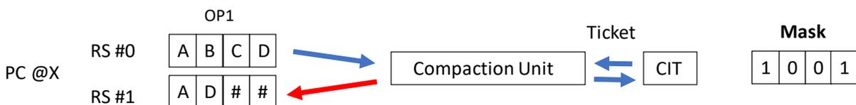
Figure 4.5: Compaction phase for one compactable instruction with a mask density of 50%.
