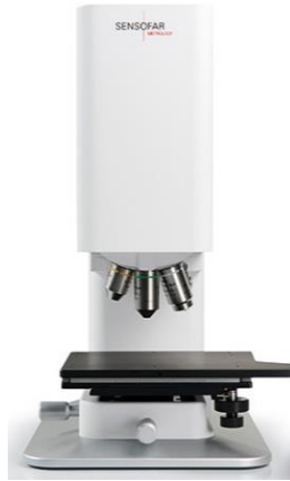
Figure 3.6 S lynx. White light confocal microscope.
