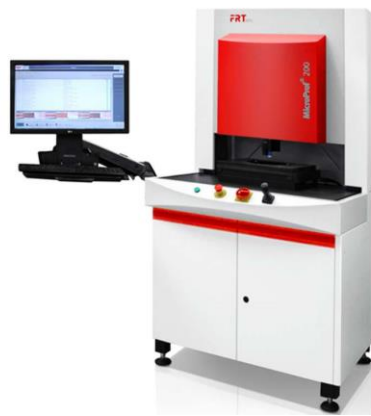
Figure 3.5 FRT Microprof 200. Chromatic confocal microscope.
