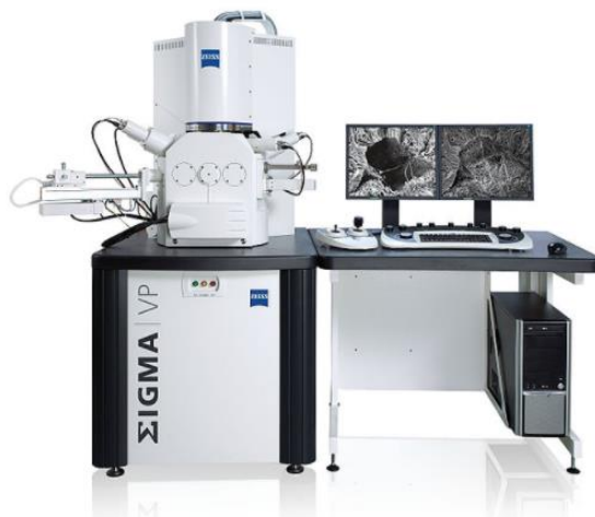
Figure 3.7 Zeiss Sigma 300 VP. Scanning electron microscope.
