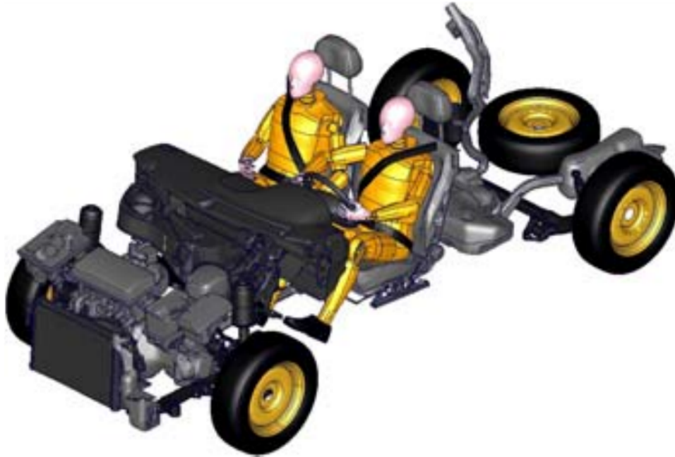
FIGURE 1.3 The 2003 Opel Astra model with dummies, controls, restraint systems and fuel tank. Source: (Böttcher, Frik, and Gosolits, 2005)
