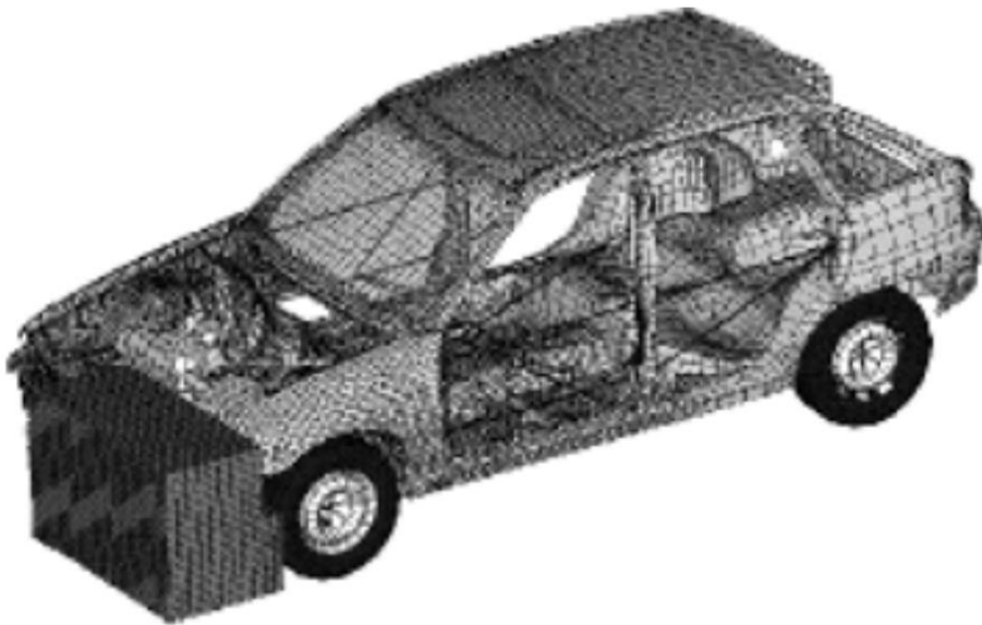
FIGURE 1.2 The 1990 Opel Astra front impact model. Source: (Böttcher, Frik, and Gosolits, 2005)
