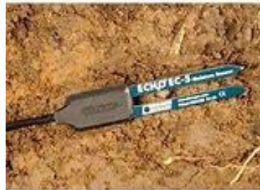
Figure 7. Datalogger (left) and ECH2O EC-5 Soil moisture sensor (right) used to determine soil humidity. Every datalogger can connect up to 5 sensors ( www.metergoup.com ).
