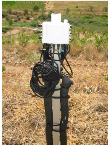
Figure 6. Installation of water soil sensors in each vineyard (Site 1 to Site 5). Datalogger. ( www.metergoup.com ).
