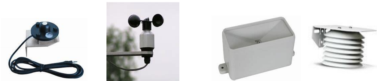
Figure 3. Pyranometer, Anemometer, Pluviometer and humidity and temperature sensors. Adapted by (www.metergoup.com).
