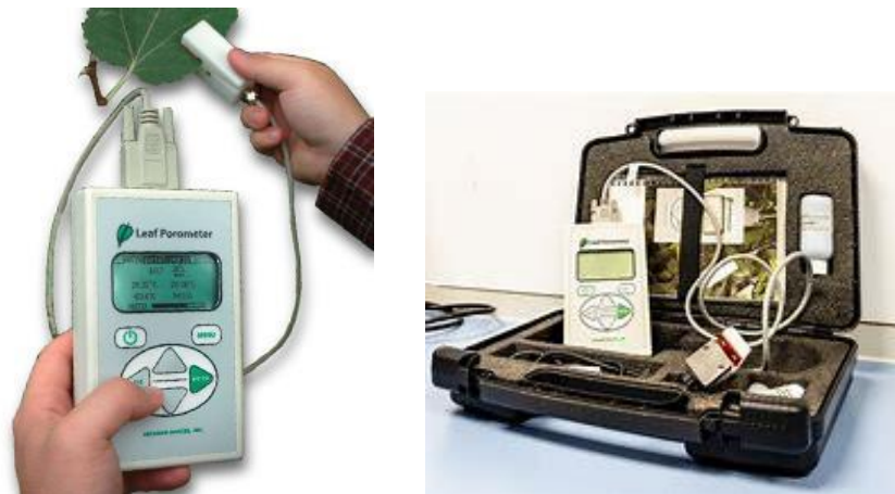
Figure 13. The steady state SC-1 Decagon® Leaf Porometer consists of a hand-held enclosure with a cable connected to a leaf-clip sensor. The final reading appears on the display in terms of either conductance or resistance. Saved data can download to a PC using an RS232 cable and download utility software. ( www.metergoup.com )
