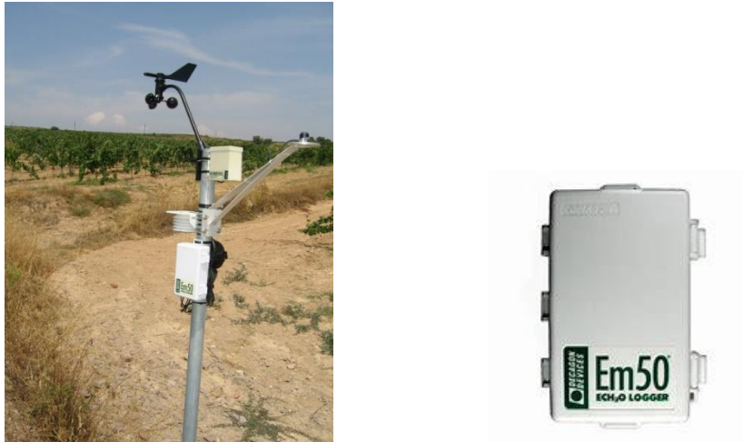
Figure 2. Installation of weather stations in each vineyard (Site 1 to Site 5). Datalogger (right).
