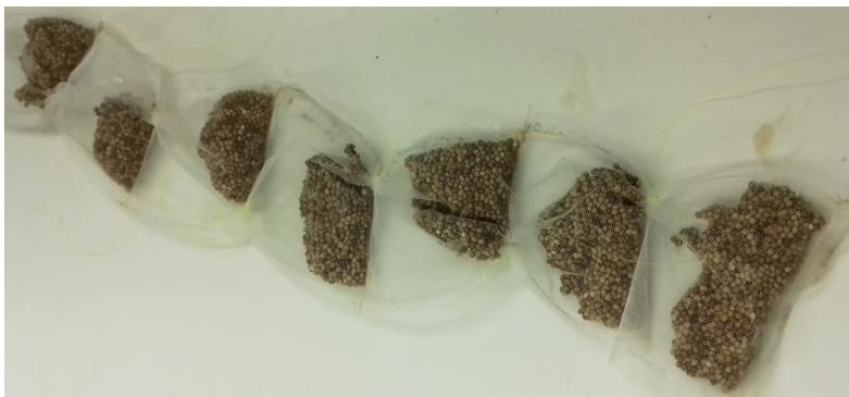
Figure S5.2: Bags with PVA beads. Each MBBR was filled with polyvinyl alcohol (PVA) beads (Kuraray Aqua Co, Ltd., Tokyo, Japan), contained in bags made from fine fishnet material and kept in suspension by the aeration and liquid recirculation. The bags prevented the beads from entering the recirculation loop and from clogging/covering the aeration stones.
