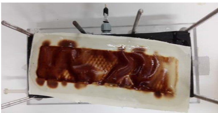
Figure S4.3: Anion exchange membrane after two days of operation.
