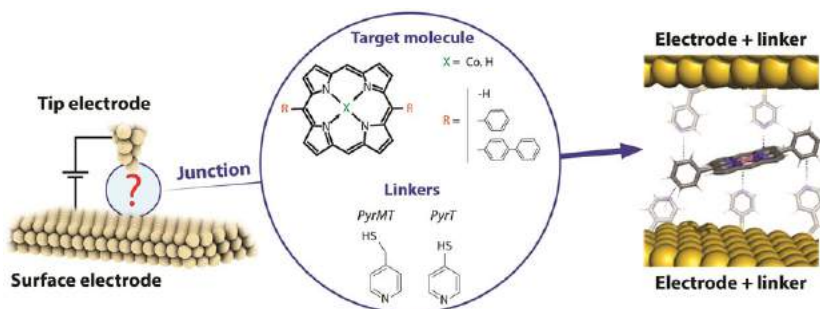
Figure 2.5. Summary of the nanojunctions studied to resolve the supramolecular scenario of CoDPP molecular junctions. 23
