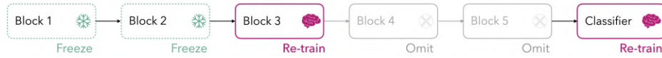
Figure 12.2: Proposed architecture for fine-tuning a VGG-19 according to the main blocks of the original network.
